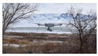
With its leading endurance and quick deployment ability, Lockheed Martin's Indago 3 is a military-grade, all-weather, group 1 quadrotor unmanned aircraft system. Credit: Lockheed. Integration of a transponder for sense and avoid; Martin
