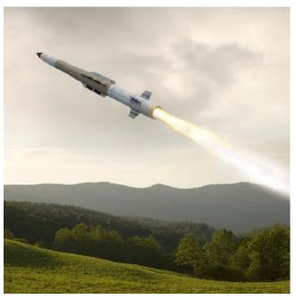
The PAC-3 MSE's revolutionary two-pulse solid rocket motor provides increased performance in both altitude and range while employing the same proven Hit-to-Kill technology that the PAC-3 CRI missile uniquely brings to the Patriot system.
