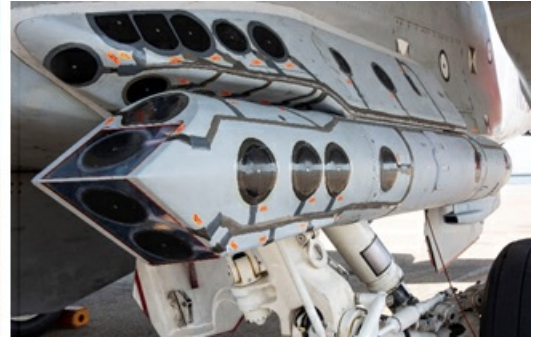
Sniper ATP is pictured on Weapon Station 5 of the F/A-18E/F during the first flight tests in March. NAVAIR Public Release SPR 2021-261 Distribution Statement A - Approved for Public release: distribution is unlimited. (photo credit: Boeing and U.S. Navy)
