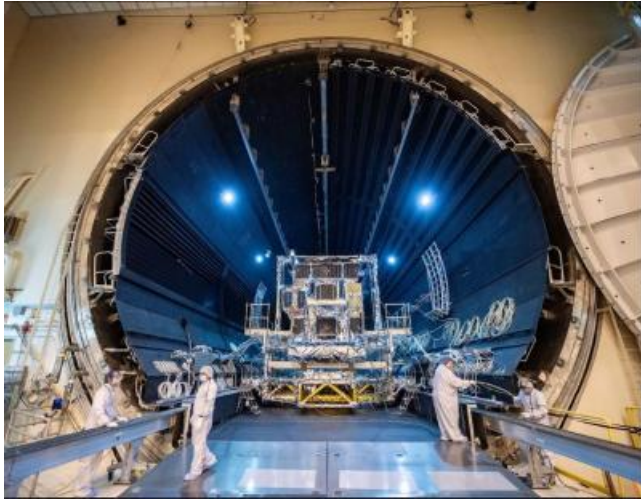
Lockheed Martin's SBIRS GEO-5 satellite, the first military space satellite built on a modernized LM 2100™ bus, recently completed Thermal Vacuum (TVAC) environmental testing.
