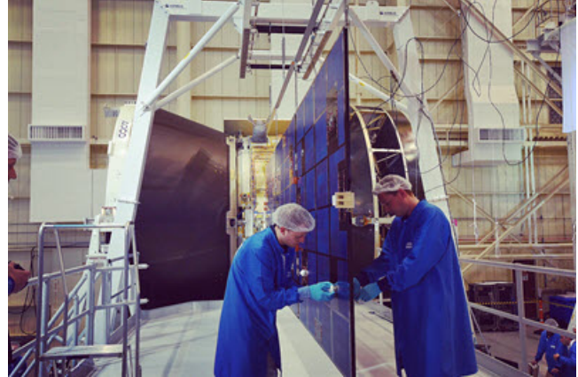
The Roving solar array simulator is used on the Orion, pictured here in a solar array deployment test (NASA image).
