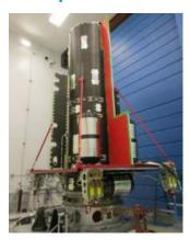
Lockheed Martin has completed the propulsion subsystem for the first modernized A2100 satellite. The hybrid chemical and electrical propulsion subsystem was built at Lockheed Martin's facility in Stennis, Mississippi and shipped to Denver, Colorado. Lockheed Martin has completed the propulsion subsystem for the first modernized A2100 satellite. Integral to the spacecraft, the subsystem helps raise the satellite into orbit after launch and keeps it on station throughout its mission life.
