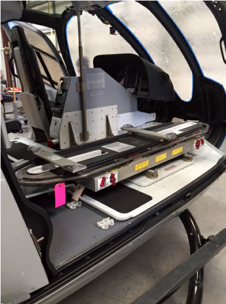
LifePort medical interior for the H130 aircraft.
