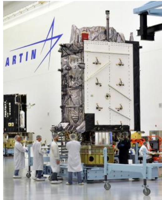
The GPS III Non-Flight Satellite Testbed (GNST) completed a series of high-fidelity pathfinding events which validate the process and facility for space vehicle integration checkout.
