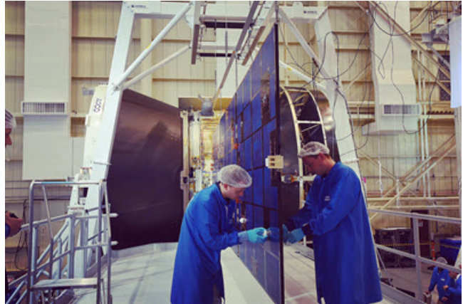
The Rovsing solar array simulator is used on the Orion, pictured here in a solar array deployment test (NASA image).
