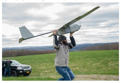
In April 2019, AFRL's Advanced Power Technology Office completed the acceptance test demonstration of Condor in Owego, NY. This demo proved the TRL 8, Group 1 UAS is ready to transition to the warfighter. Credit: Lockheed Martin
