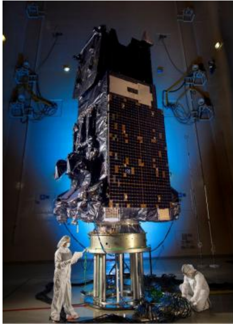
Lockheed Martin's SBIRS GEO-5 satellite, the first military space satellite built on a modernized LM 2100™ combat bus, built in record speed, is ready for a 2021 launch.
