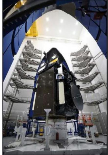
*Lockheed Martin's sixth Advanced Extremely High Frequency (AEHF-6) protected communications satellite is encapsulated in its protective fairings ahead of its expected March 26 launch on a United Launch Alliance Atlas V rocket.*
