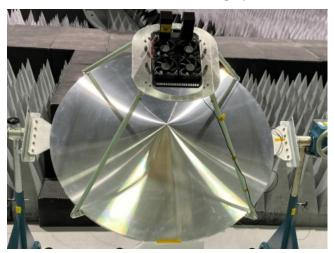
LITTLETON. Colo... Aug. 23, 2021 -Lockheed Martin (NYSE: LMT) has invented a new type of satellite dish technology with a wide range of use on satellites and ground terminals, including space-based 5G. The Wide Angle ESA Fed Reflector (WAEFR) antenna is a hybrid of a phased array Electronically
