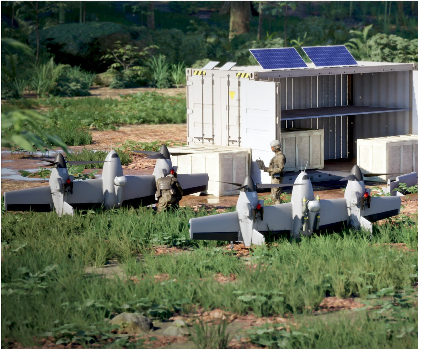
Four ready-to-fly autonomous Nomad 100 aircraft in a single 20-foot container enabling rapid deployment and sustainment. Rendering courtesy of Sikorsky, a Lockheed Martin company.
