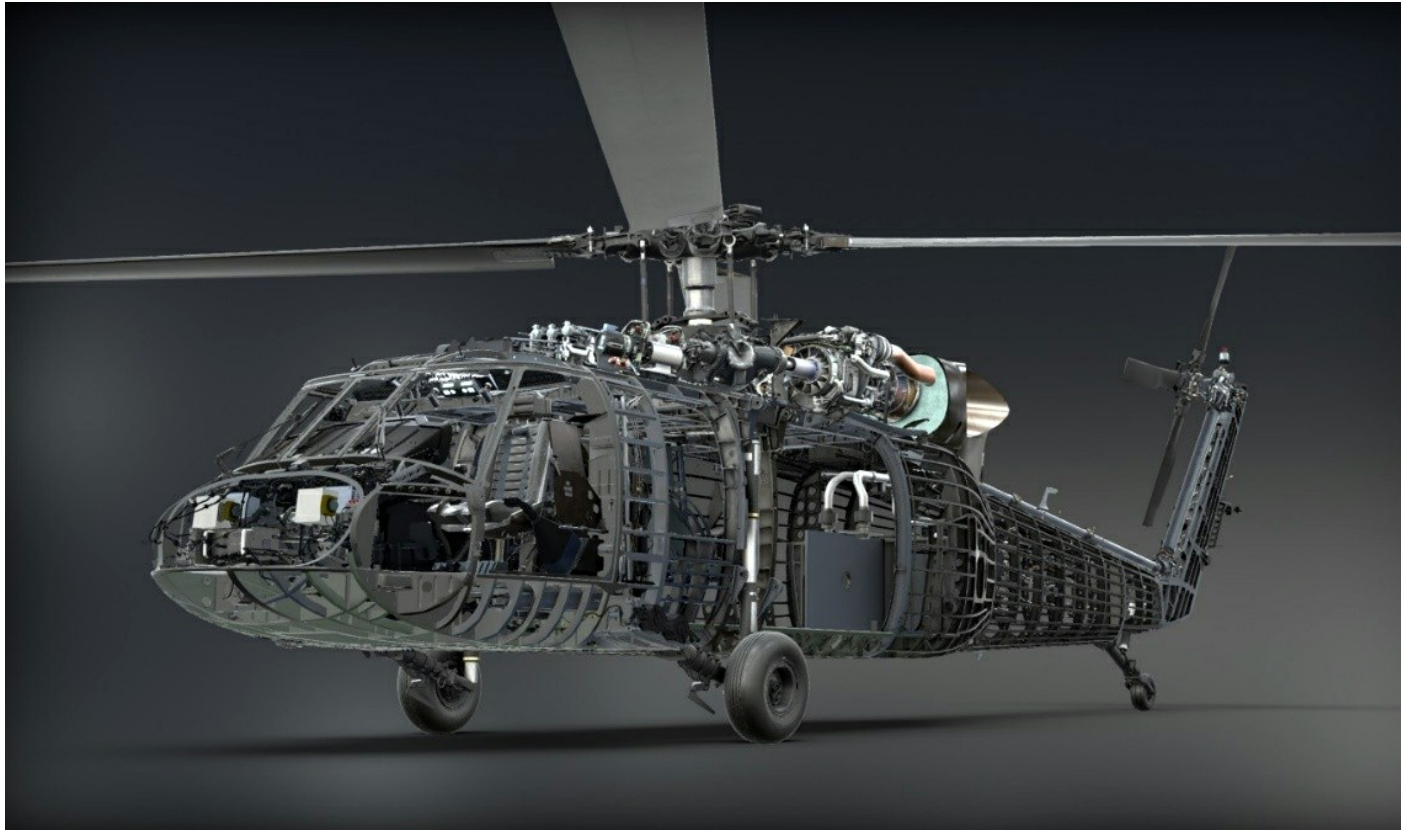
Lockheed Martin's S-70i Black Hawk virtual maintenance trainer provides interactive 3D simulations of maintenance tasks and is one of a family of high-fidelity, synthetic training devices currently available. Image courtesy Lockheed Martin.
