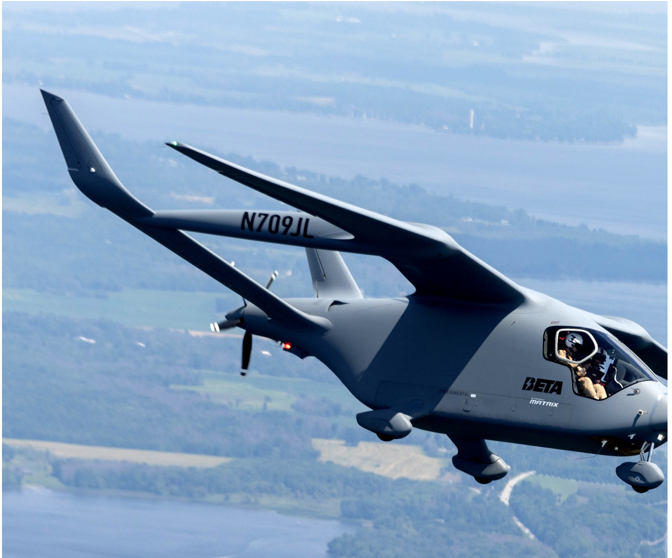
BETA successfully integrated Sikorsky's MATRIX™ autonomy suite on BETA's ALIA CTOL (CX300) as a testbed for BETA's MV250 aircraft initiative. Photo courtesy Sikorsky, a Lockheed Martin company.
