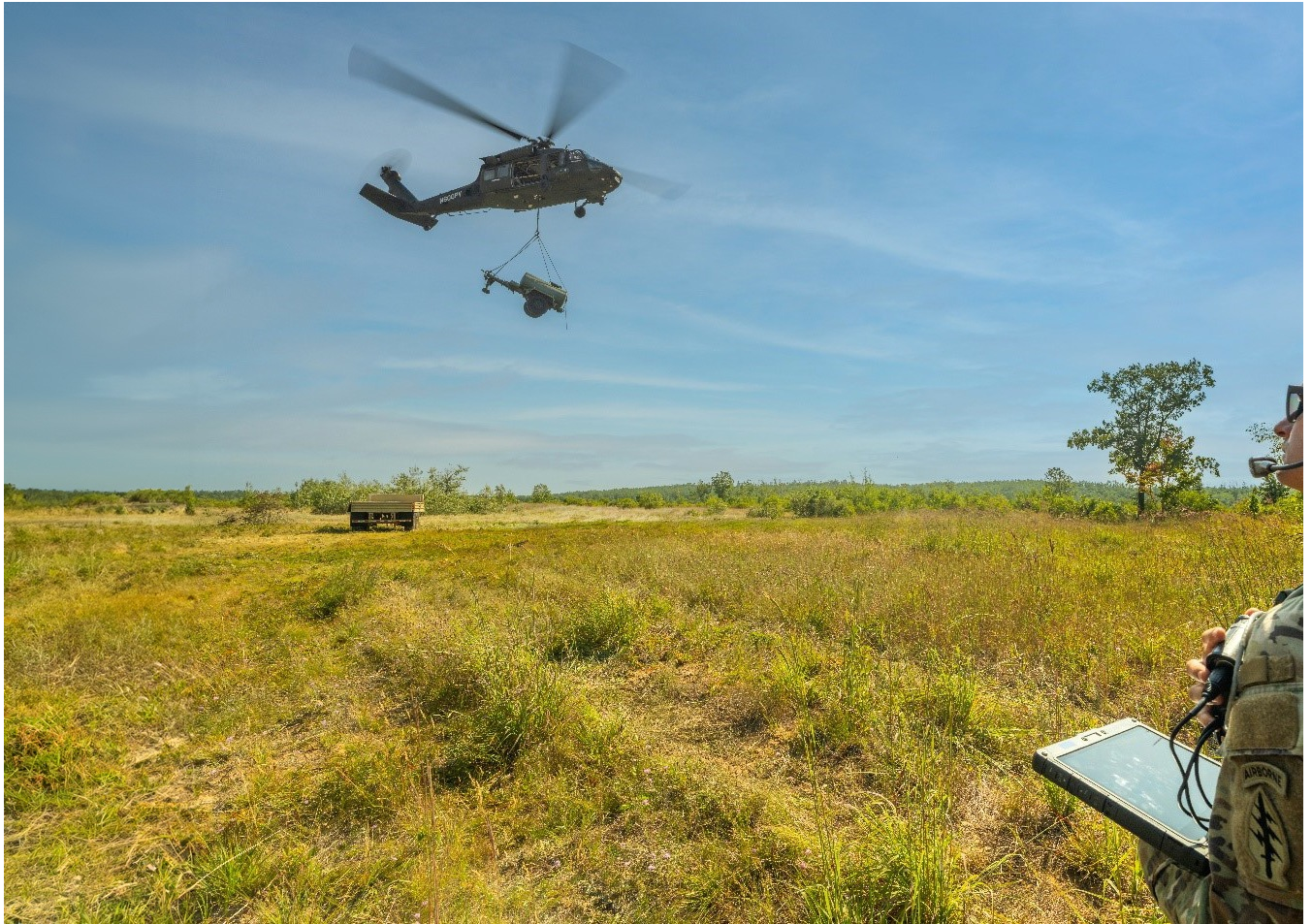
U.S. Army National Guard Sgt. uses a tablet to command the Sikorsky OPV Black Hawk to autonomously transport a 2,900-pound water buffalo sling load for the first time during Northern Strike in Michigan. Photo courtesy Sikorsky, a Lockheed Martin company.
