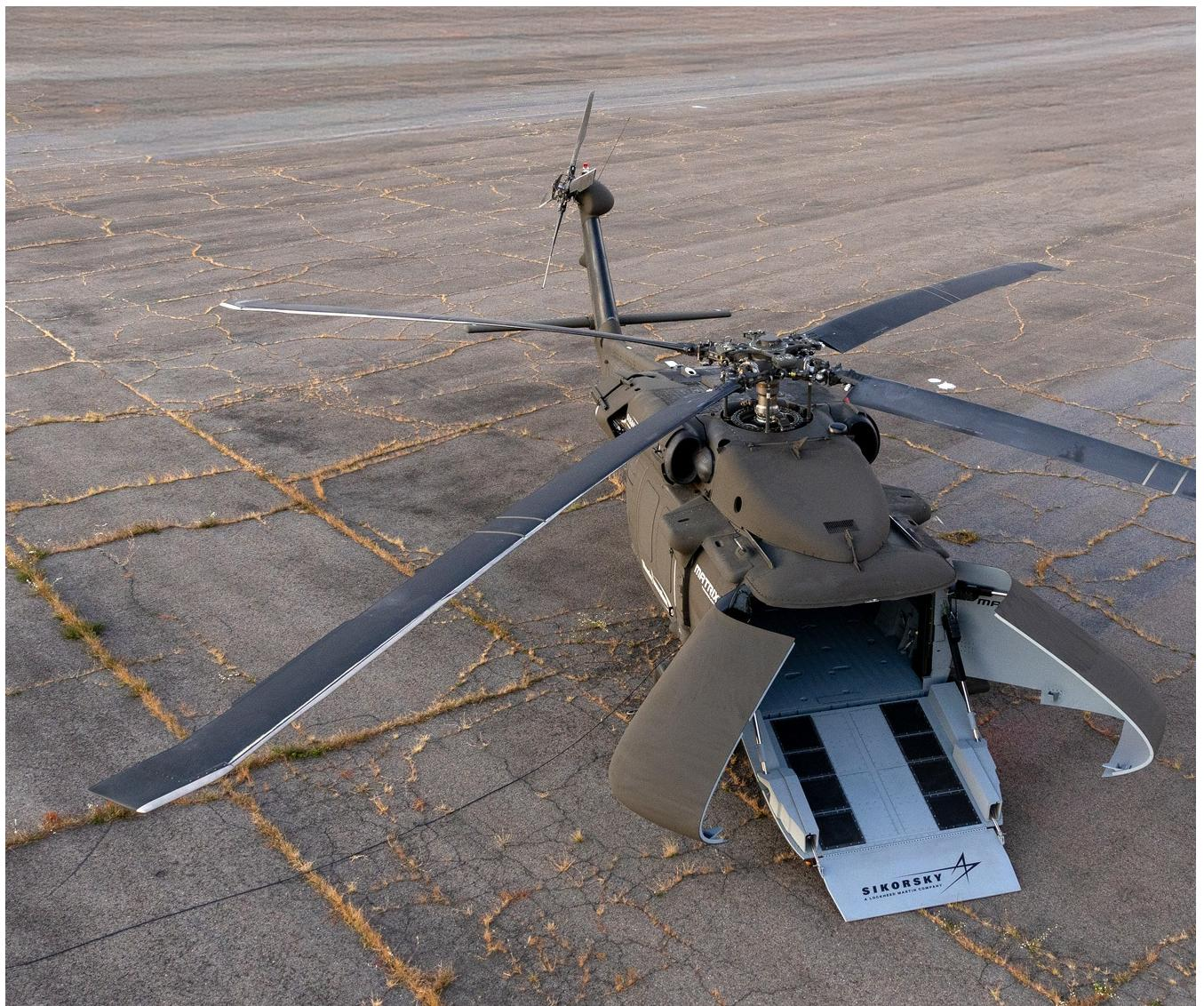
By removing the cockpit, seats and crew stations, the Sikorsky S-70UAS™ U-Hawk™ helicopter becomes the first fully autonomous Black Hawk helicopter. Photo courtesy, Sikorsky, a Lockheed Martin company.
