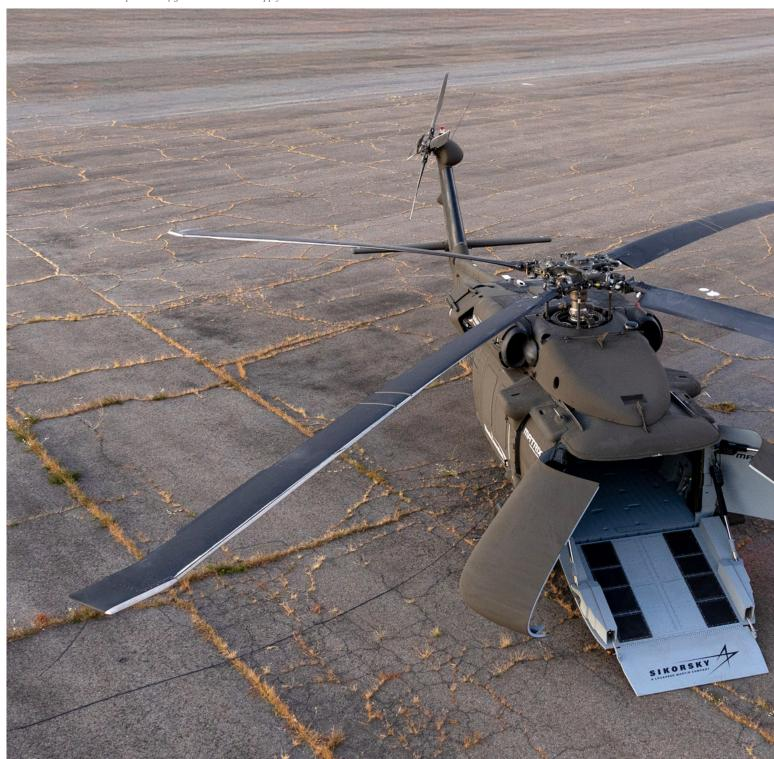
By removing the cockpit, seats and crew stations, the Sikorsky S-70UAS<sup>TM</sup> U-Hawk<sup>TM</sup> helicopter becomes the first fully autonomous Black Hawk helicopter. Photo courtesy, Sikorsky, a Lockheed Martin company.
