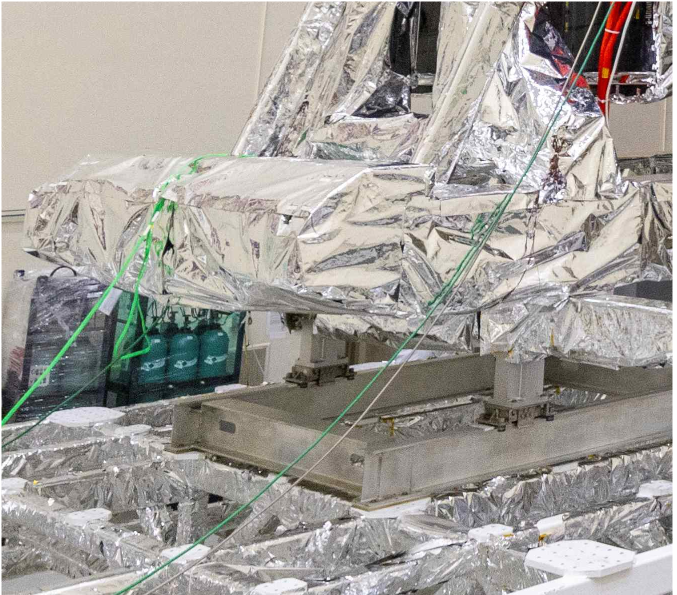
The first Next-Gen OPIR GEO satellite has completed environmental testing (thermal vacuum testing pictured above).
