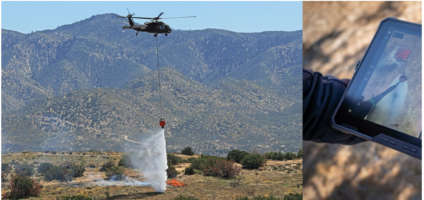
A Black Hawk® helicopter equipped with Sikorsky MATRIX™ and Rain autonomy drops water onto a staged burn in Calif., April 24. A tablet shows an active suppression task with the fire location and suppression plan visible. Photos courtesy of Rain.
