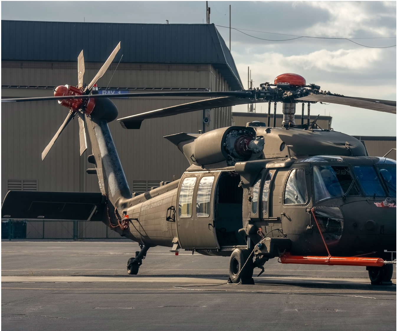
Sikorsky started ground runs on a UH-60M Black Hawk equipped with two Improved Turbine Engines. This engine increases the Black Hawk's combat capabilities. Photo courtesy Sikorsky, a Lockheed Martin company. ©Lockheed Martin Corporation.
