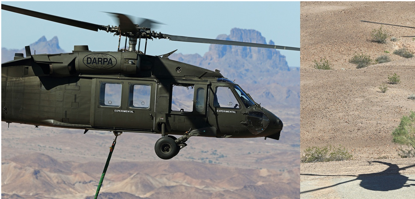
Sikorsky's Optionally Piloted Black Hawk will help the U.S. Marine Corps test flight autonomy for resupply in contested battlespace. Photo: Uncrewed aircraft with external load at U.S. Army Yuma Proving Ground in 2022. Sikorsky, a Lockheed Martin company.
