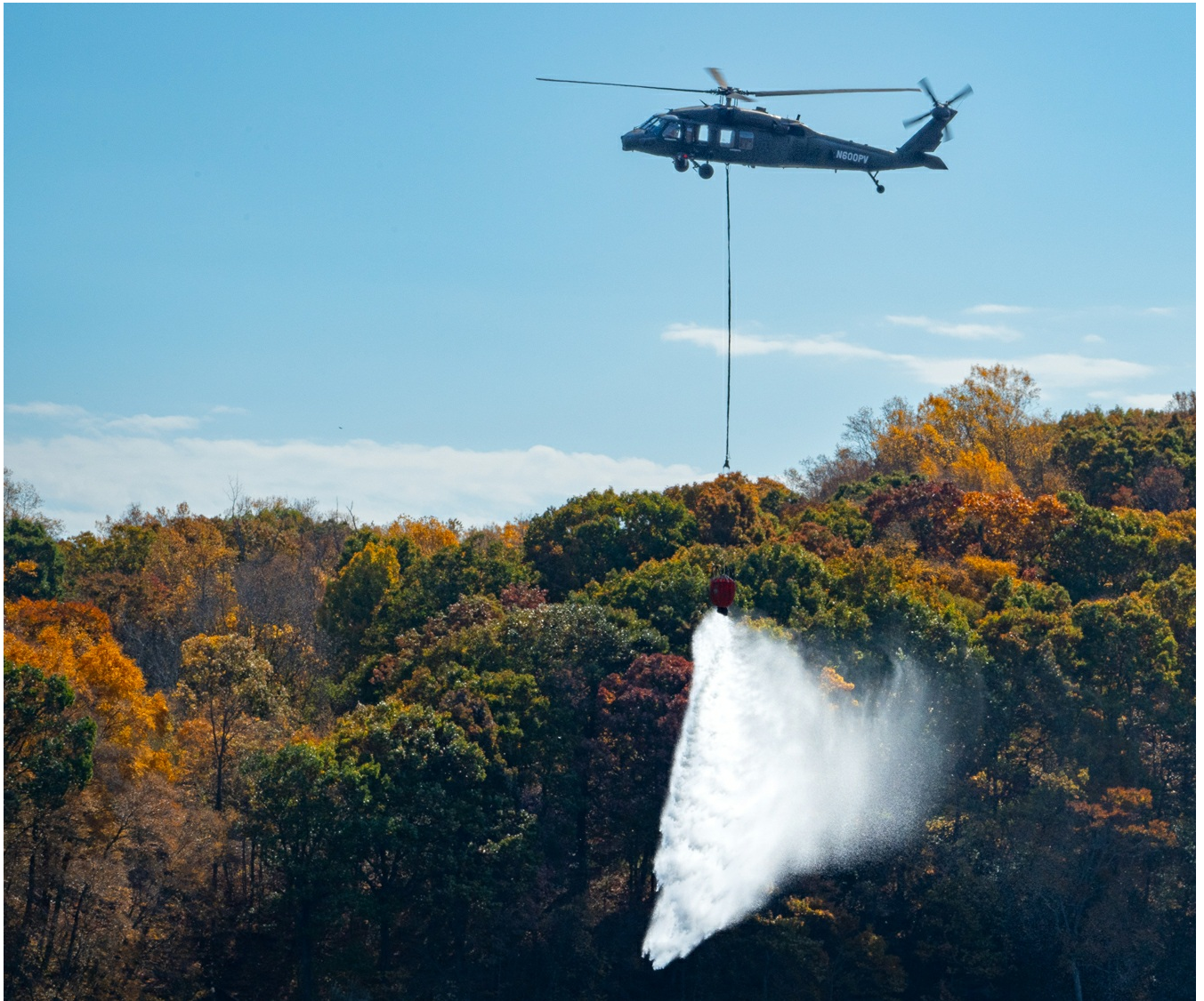
An autonomous Black Hawk® helicopter demonstrates an aerial water drop Oct. 29 in Connecticut. A Wildfire Mission Autonomy System developed by Rain commanded the autonomous aircraft to launch, find and suppress the fire. Photos courtesy of Rain.
