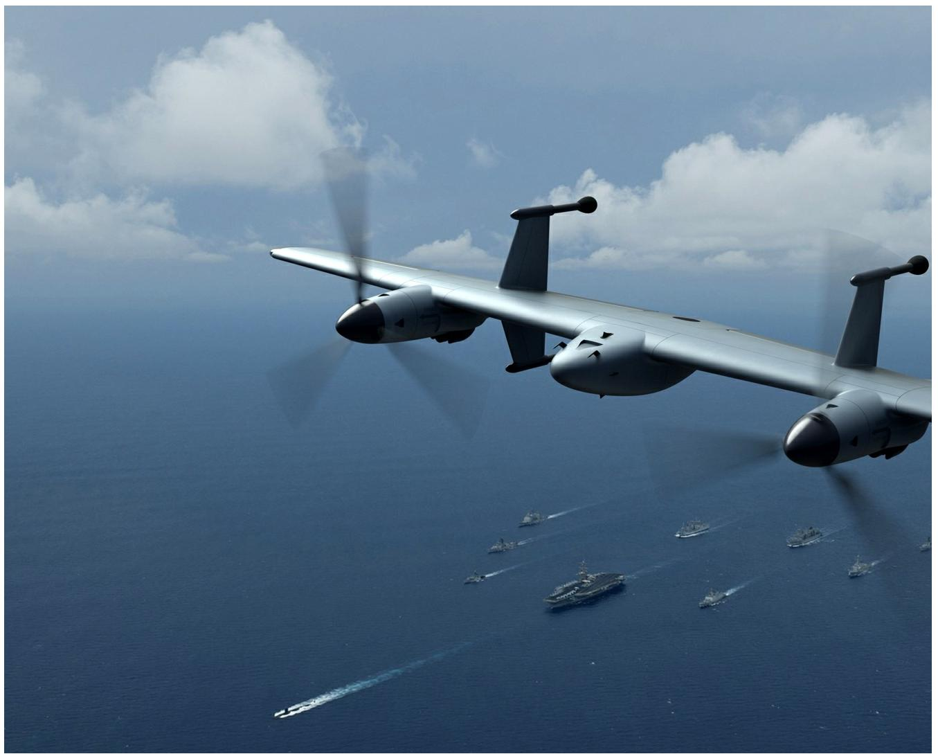
*Sikorsky is flight testing a rotor blown wing tail sitter VTOL UAS. Prop rotors, electrification, and autonomy are key enabling technologies for efficient vertical and horizontal flight. © 2024 Lockheed Martin Corporation. All Rights Reserved.*
