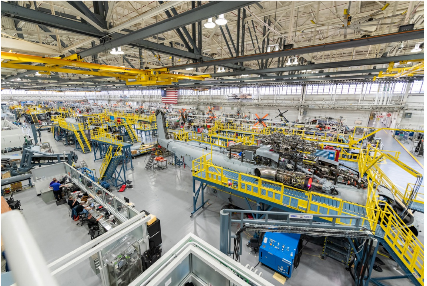
Sikorsky employees building CH-53K® aircraft utilizing 3-D work instructions, new titanium machining centers with multi-floor ergonomic platforms.
