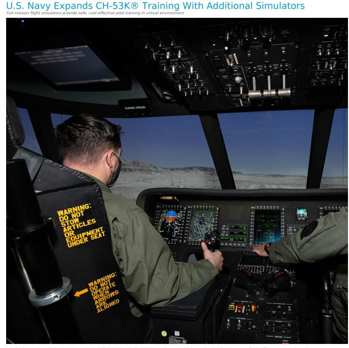
Marine Corps aviators in the CH-53K Containerized Flight Training Device (CFTD) experience a highly immersive virtual environment allowing flight crews to train on the full scope of Marine Corps heavy lift missions, including external lift operations.
