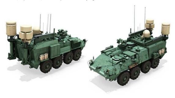
Lockheed Martin will integrate the Terrestrial Layer System prototype onto the U.S. Army's Stryker vehicles. Photo courtesy Lockheed Martin
