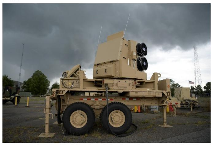
Sentinel A4 is a high-performance missile defense radar that will provide significant improvements to existing capability against cruise missiles, unmanned aerial systems, rotary wing and fixed wing threats. Photo courtesy Lockheed Martin
