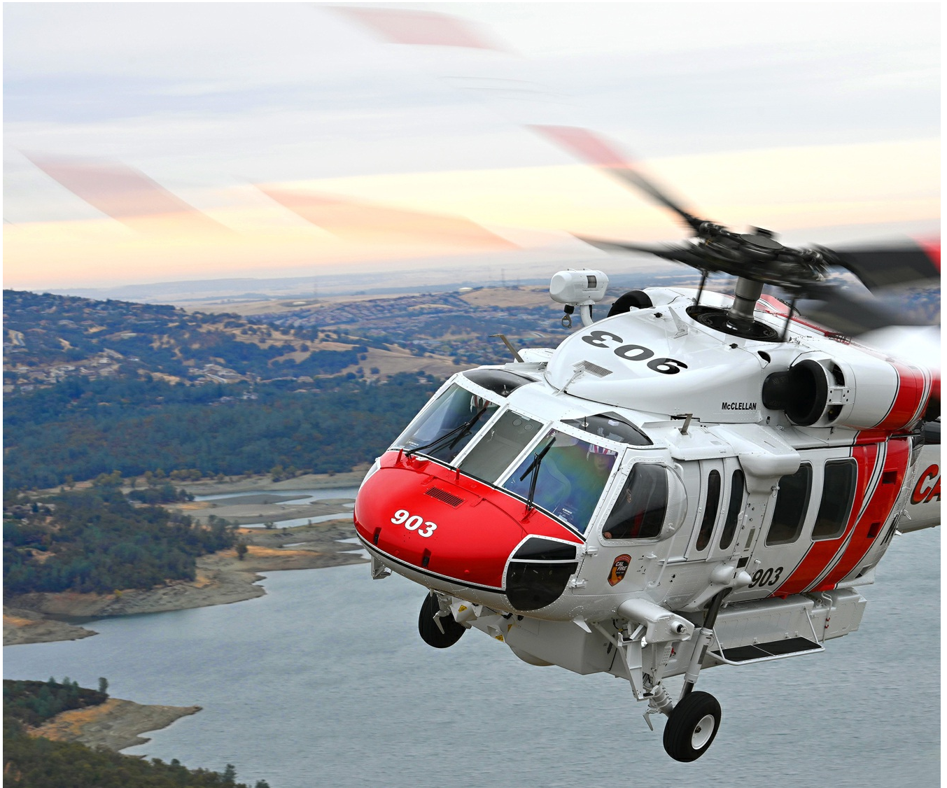
An S-70 FIREHAWK helicopter operated by CAL FIRE can transport firefighters, drop water on wildfires from its 1,000-gallon (3,785 liter) belly tank, and perform hoist rescues.
