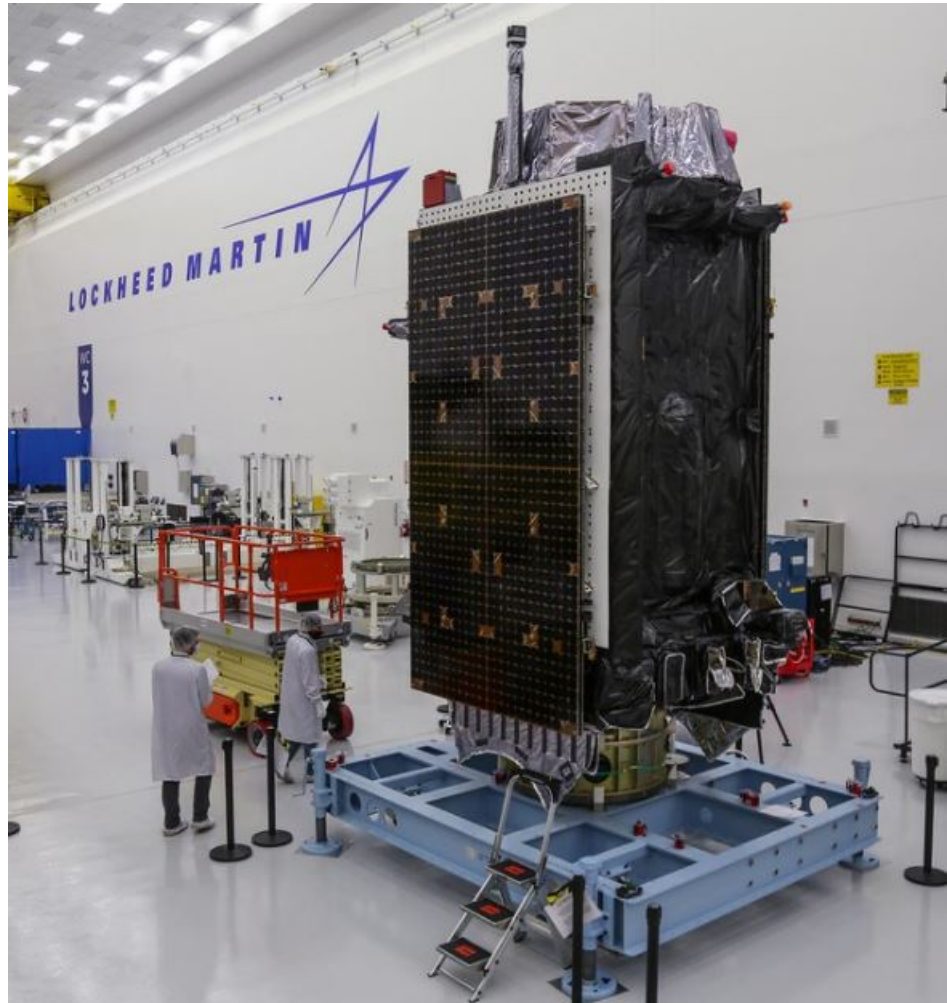
The fifth Lockheed Martin-built GPS III satellite at Lockheed Martin's production facility prior to its June 17 launch.
