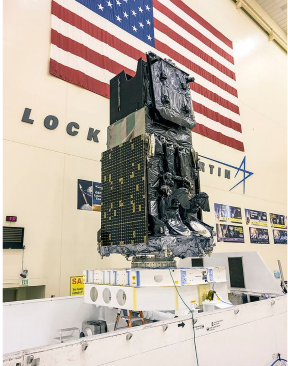
Lockheed Martin's SBIRS GEO-5 missile warning spacecraft is the first military space satellite built on a modernized LM 2100 Combat Bus™ space vehicle.
