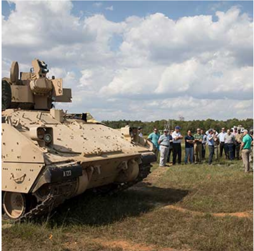
A U.S. Army-led MAPS team takes to the field at Redstone Test Center in 2019 to demonstrate a layered defense capability to defeat threats. This was the first use of the base kit in a ground vehicle, in this case a Bradley. Photo credit: U.S. Army.
