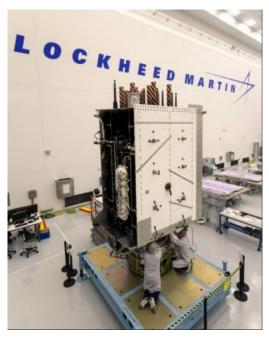
Lockheed Martin's GPS III Space Vehicle 03, launched today, as it appeared in the company's cleanroom GPS III Processing Facility.
