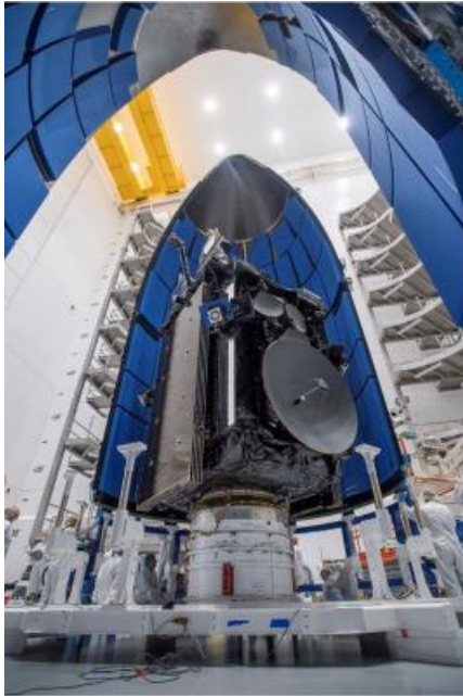
The U.S. Air Force's fifth Advanced Extremely High Frequency (AEHF-5) protected communication satellite encapsulated prior to launch.
