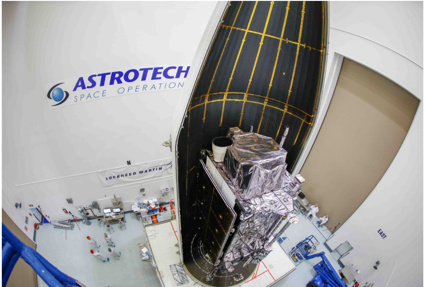
The U.S. Air Force's second Lockheed Martin-built GPS III satellite is encapsulated for launch.
