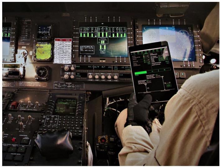
The iFly Sikorsky app gives 5-70i pilots and mission planners a quick and easy method to configure the aircraft for flight.
