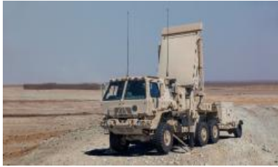
The multi-mission Q-53 protects troops in combat by detecting, classifying, tracking and identifying the location of enemy indirect fire.
