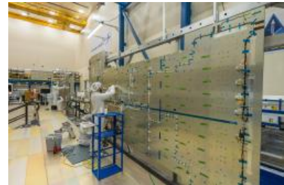
Lockheed Martin technicians begin assembly on the JCSAT-17 commercial communications satellite in a clean room near Denver.
