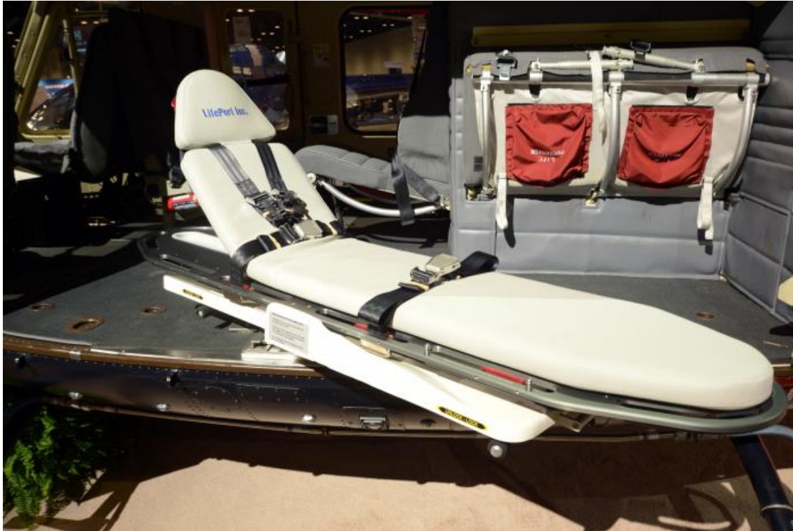
LifePort machined sled in Bell 412 helicopter.
