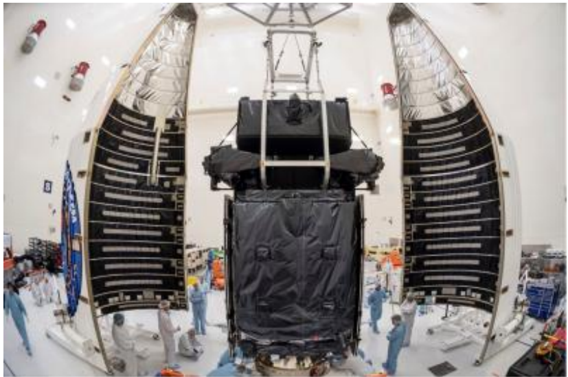
The U.S. Air Force's SBIRS GEO Flight-4 satellite, built at Lockheed Martin's Sunnyvale, California satellite manufacturing factory, was encapsulated on Jan. 9.
