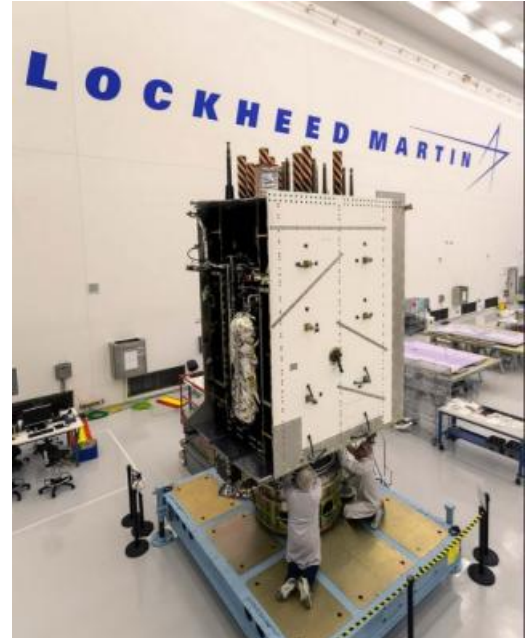
The U.S. Air Force's third GPS III satellite, GPS III SV03, is now fully integrated and ready to begin environmental tests. Lockheed Martin is in full production on ten contracted GPS III satellites at its GPS III Processing Facility near Denver.
