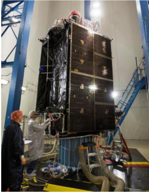
The U.S. Air Force's second GPS III satellite, GPS III SV02 (above), recently completed acoustic testing, which simulates the stress the satellite will experience during launch.
