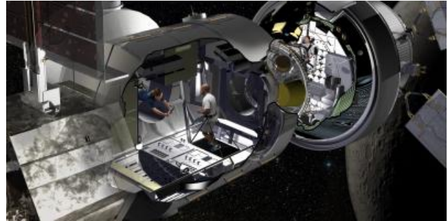
Lockheed Martin artist rendering of the NextSTEP habitat docked with Orion in cislunar orbit as part of a concept for the Deep Space Gateway.
