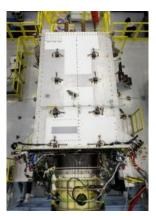
The U.S. Air Force's second GPS III satellite, GPS III SV02, is fully integrated and ready for environmental tests this summer at Lockheed Martin's GPS III Processing Facility.
