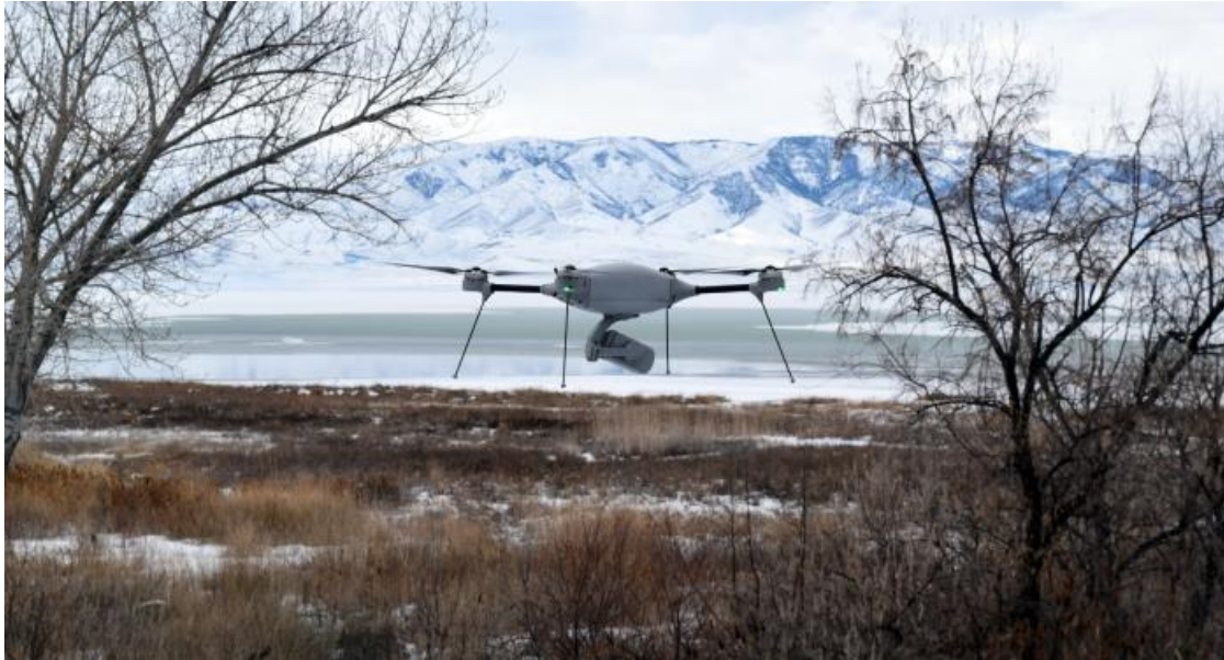
Indago 3 is a military-grade, all-weather quadrotor UAS equipped with TrellisWare Technologies software to provide a long-range, secure ISR platform for sensitive military operations. Photo courtesy Lockheed Martin.
