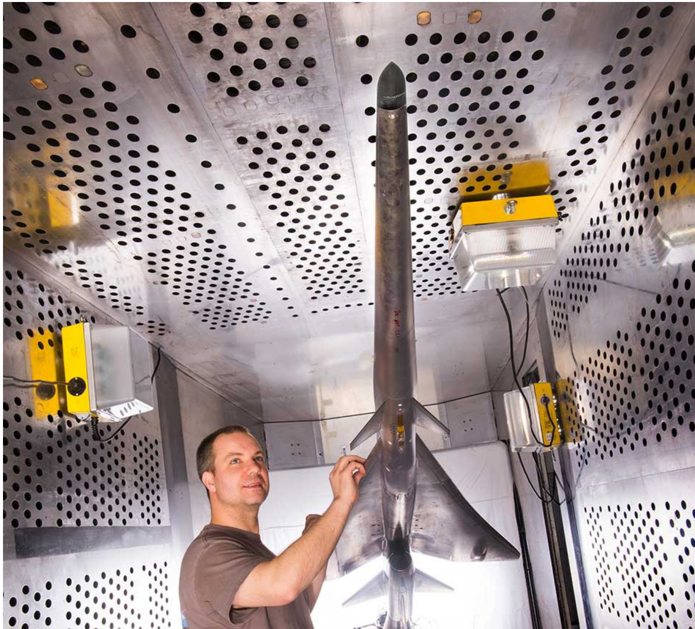
Mechanical technician Dan Pitts prepares the model for wind tunnel testing. Credit: NASA
