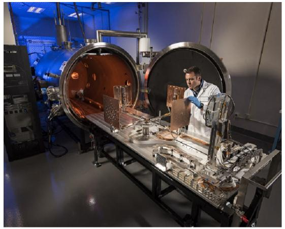
Lockheed Martin's new Space Plasma and Radiation Center (SPARC) features one of the world's few atomic particle accelerators that the facility will use to mimic the sun's effects on space instruments.
