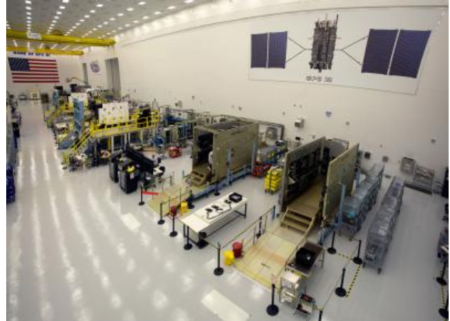
GPS III satellites in production at Lockheed Martin's GPS III Processing Facility near Denver.
