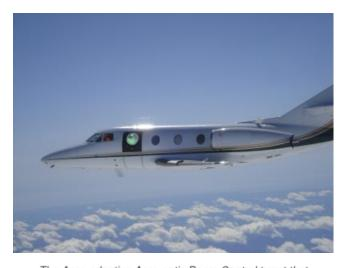
The Aero-adaptive Aero-optic Beam Control turret that Lockheed Martin is developing for the Defense Advanced Research Projects Agency and the Air Force Research Laboratory has completed initial flight testing. (Photo: Air Force Research Laboratory.)
