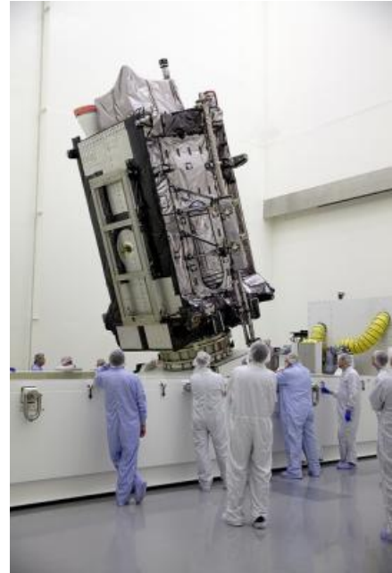
Lockheed Martin's GPS III Non-Flight Satellite Testbed (GNST), a full-sized, functional GPS III satellite prototype, communicated via cross-links with Air Force flight-like hardware simulators for the GPS IIR, GPS IIR-M, and GPS IIF satellites.
